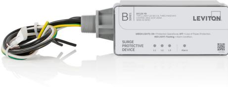
B Series Type 2 Surge Panel, 208Y/120 VAC, Three Phase WYE, Max Surge Current Rating of 65kA per Mode/130kA per Phase, 200kA Short Circuit Current Rating (SCCR), 20kA I-nominal ( $I_n$ ) Rating, NEMA 4X Rated Enclosure, Thermally Protected MOVs, VPR Performance Data = L-N: 700, L-G: 700, N-G: 600, L-L: 1200, Maximum Continuous Operating Voltage (MCOV): 150V /300V, Plastic Enclosure, LED Status Monitoring, Audible Alarm, UL 1449 Listed, UL 1283 EMI/RFI Filtering, Approximate Lead Length = 18"
