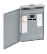
Load center, QO, 1 phase, 20 spaces, 24 circuits, 100A convertible main breaker, PoN, NEMA3R, UL
